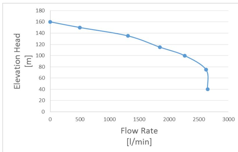
Fig. 6. Characteristic curve of a FP 24/8 type pump (source: Authors’ design)
