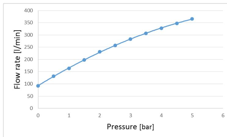
**Fig. 4.** The flow rate changes of the first stream (Source: Illustrated by the Authors)
