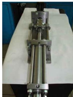
Testing of the sealing elements has been conducted on a stand from the Laboratory of servo-technique at IHP – Bucharest; the test stand has been adjusted in order to meet the requirements of the diagram in fig. 1.
