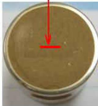
Fig. 7. Recording zone of cavitated area roughness, with the Mitutoyo apparatus
