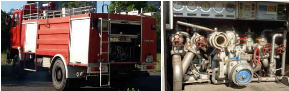
Fig. 1. Csepel-Metz TLF 24/50 heavy-duty truck fire hose and the inbuilt FP 24/8 type pump (Sources: Authors' photos)
