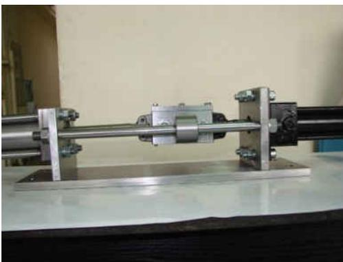
**Fig. 10.** Device for testing piston-type seals, assembled
