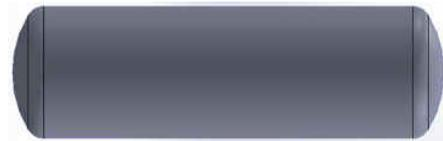
Fig. 2. The tank with ellipsoidal head covers
