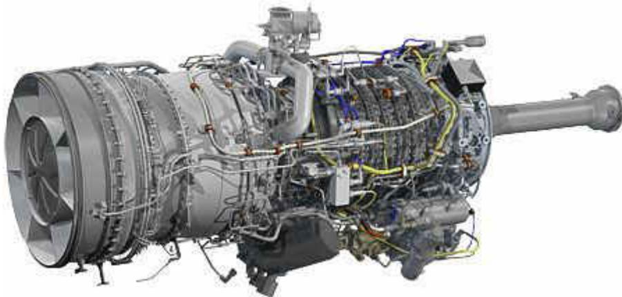
Fig. 6. Rolls Royce Tyne RM1C gas turbine [11]
