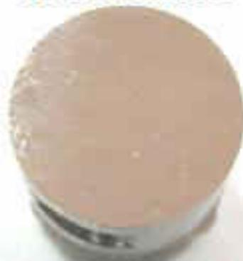
Fig. 2. The sample surface before cavitation exposure
