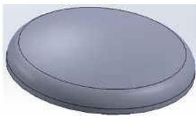
Fig. 3. The model of torospheric head cover
