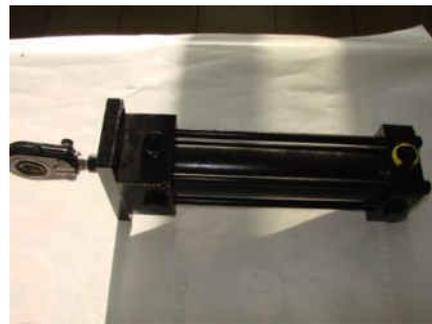
**Fig. 7.** Standard hydraulic cylinder D<sub>p</sub> 50-code CH 16U050/22-145.4.HM3.0
