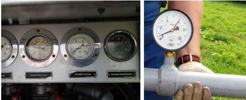
**Fig. 5.** The measured values on the Metz FP 24/8 type fire pump and the pitot tube at the moment of the cavitation (Source: Authors’ captures)
