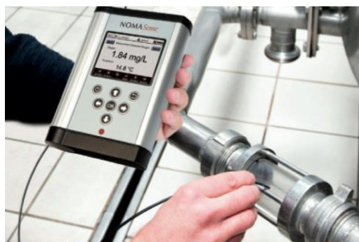
Fig. 4. Non-invasive device for measuring dissolved oxygen concentration
