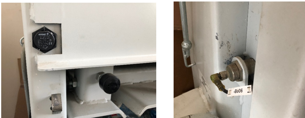
Fig. 4. Mounting detail of door switch (left) and B2 limit switch (right)
