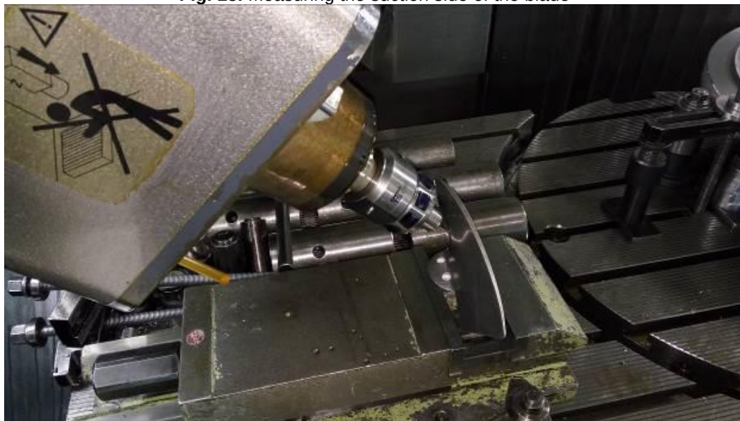
Fig. 16. Measuring the pressure side of the blade
