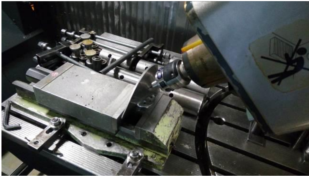
Fig. 15. Measuring the suction side of the blade
