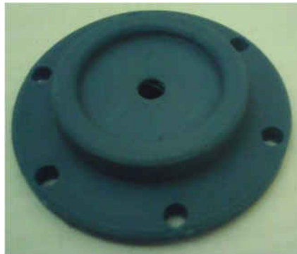
Fig. 7. Cap of a cylinder for a hydraulic or pneumatic installation slice generated parameter
