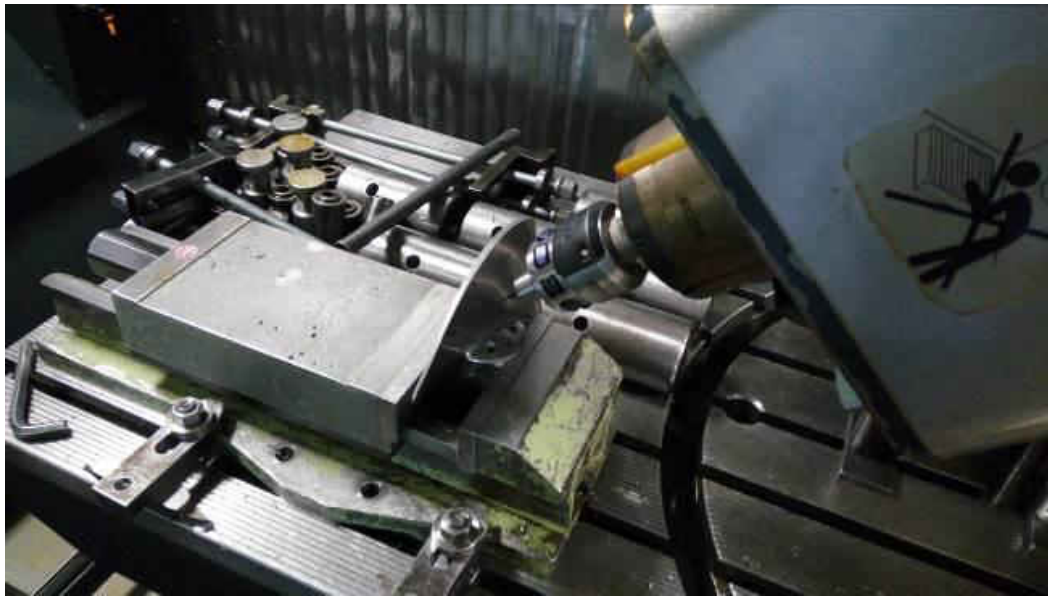
Fig. 15. Measuring the suction side of the blade
