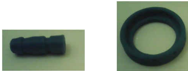
Fig. 4. Coupling pneumatic at left and printing statistic at right generated by FDM 3D printing solution
