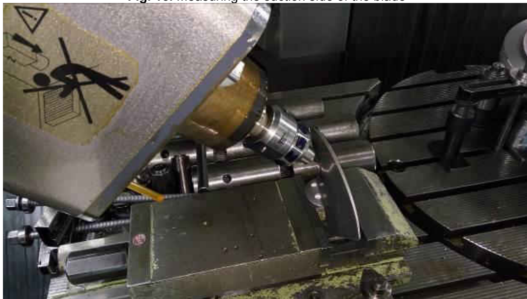
Fig. 16. Measuring the pressure side of the blade
