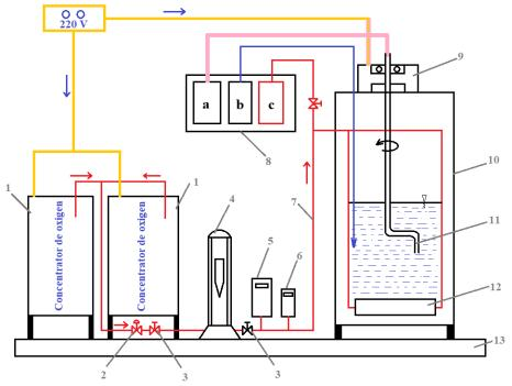
Fig. 8. Scheme of the experimental installation for researches on water oxygenation with oxygen concentrators
