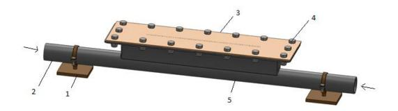
Fig. 1. Rectangular shaped fine bubble generator
