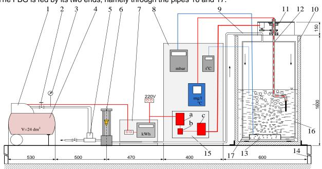
The FBG is fed by its two ends, namely through the pipes 16 and 17.
