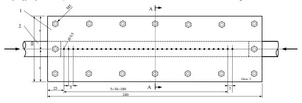
Fig. 2. Sketch of the rectangular shaped fine bubble generator perforated plate 1- orifice plate; 2- compressed air feed pipe.
