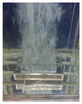
Fig. 5. Water oxygenation installation with one FBG in operation
