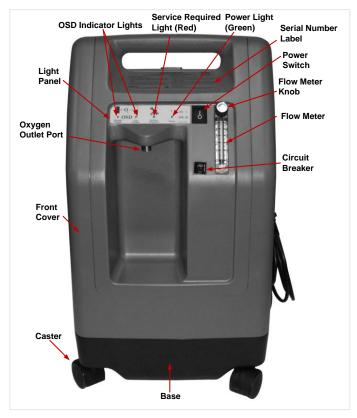
Fig. 7. Components of the DeVilbis oxygen concentrator
