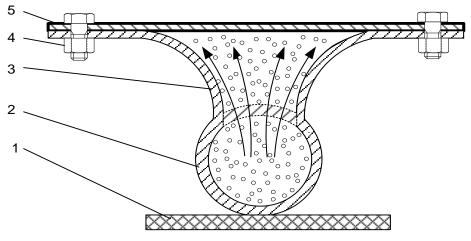
**Fig. 3.** Section from the rectangular shaped FBG. 1 – support; 2 – compressed air feed pipe; 3 – FBG body; 4 – screws for fastening the plate on the body; 5 – orifice plate.
