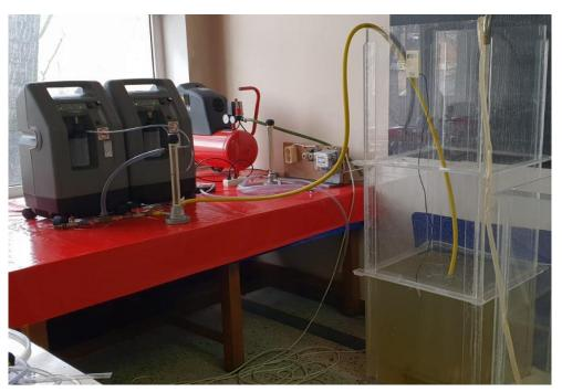
Fig. 9. Overview of the experimental installation with two oxygen concentrators
