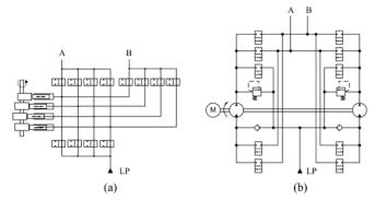
Fig. 3. (a) Two-outlet piston type DHPMS; (b) DHPMS based on fixed-displacement units [1]
