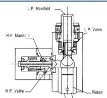
Fig. 2. Cylinder head arrangement of a digital-displacement pump-motor [2]
