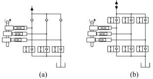
Fig. 5. (a) Piston type digital pump; (b) pump-motor [1]
