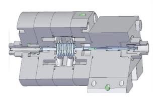
Fig. 7. CAD model of the fast switching linear valve [6]
