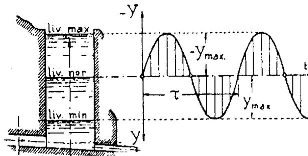
Fig. 2. Variation of the height Y to the fluid oscillations in the tank
