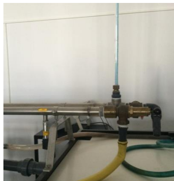
Fig. 6. Experimental stand details a) reservoir, b) piezometric tube, valves, pressure transducers, c) drive pump [2]
