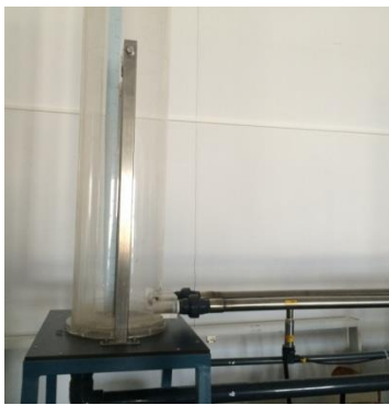
Fig. 6. Experimental stand details a) reservoir, b) piezometric tube, valves, pressure transducers, c) drive pump [2]
