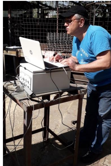
Fig. 9. Electric panel of the heat generator; programming the monitoring system for working parameters and data acquisition
