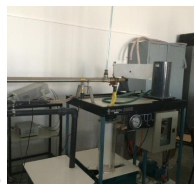
Fig. 6. Experimental stand details a) reservoir, b) piezometric tube, valves, pressure transducers, c) drive pump [2]
