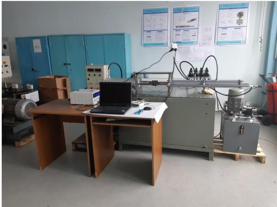
**Fig. 3.** Test stand for digital hydraulic cylinders
