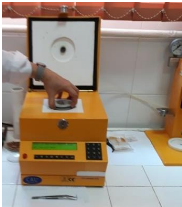
Fig. 5. Inserting the bomb calorimeter into the calorimeter
