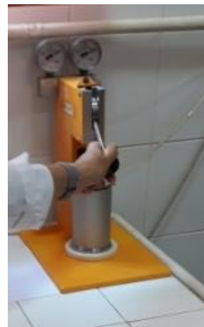
Fig. 4. Oxygen pressurization of the combustion vessel
