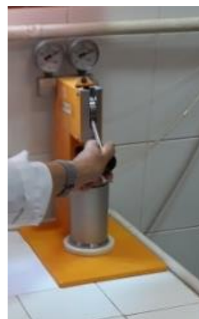
Fig. 4. Oxygen pressurization of the combustion vessel
