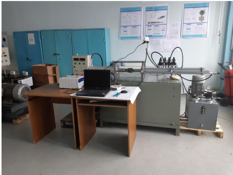
Fig. 3. Test stand for digital hydraulic cylinders
