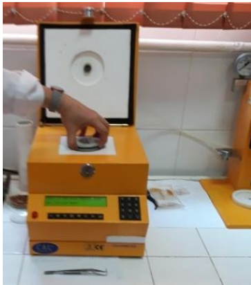
Fig. 5. Inserting the bomb calorimeter into the calorimeter
