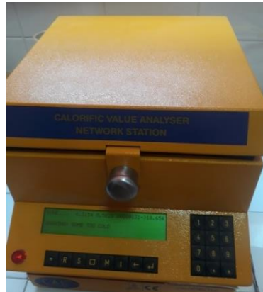
Fig. 6. Closing the calorimeter lid to start burning the biofuel sample
