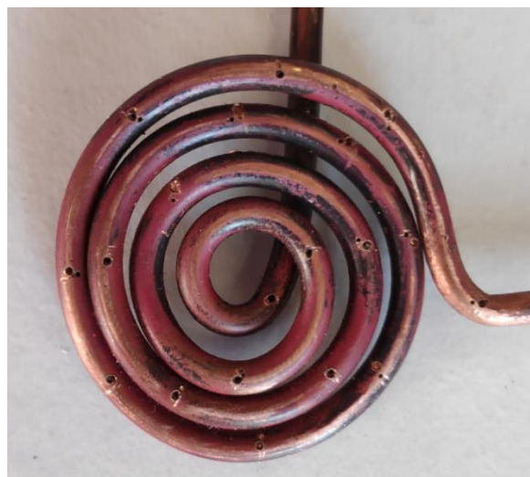
Fig. 8. Plan view of the spiral with 17 orifices \varnothing 0.3 mm
