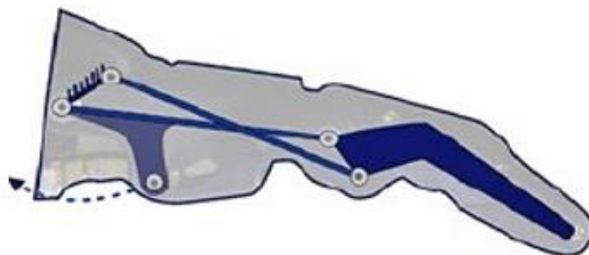
Fig. 7. Kinematic model for prosthetic finger [6]
