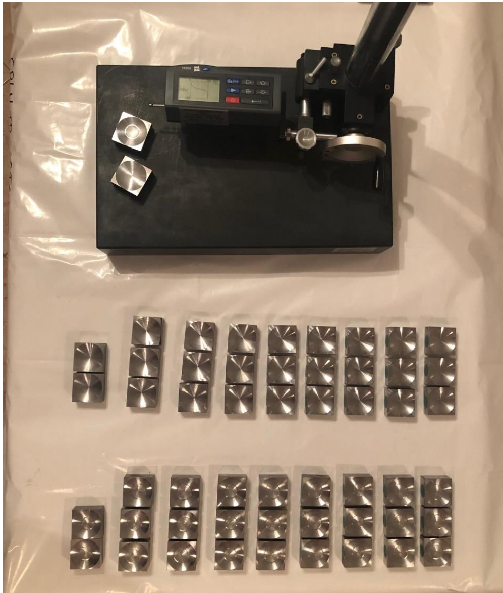
Fig. 6. The convex spherical surfaces processed with the two types of mills prepared for measurement
