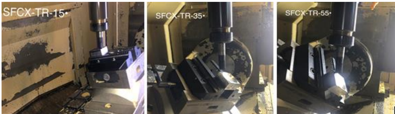
Fig. 4. Processing of the convex spherical surface with the toroidal milling in the case of the 3 types of inclinations
