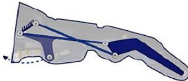
Fig. 7. Kinematic model for prosthetic finger [6]
