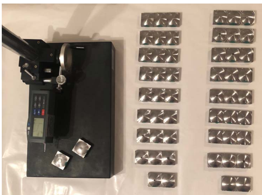
Fig. 6. The concave spherical surfaces processed with the two types of mills prepared for measurement
