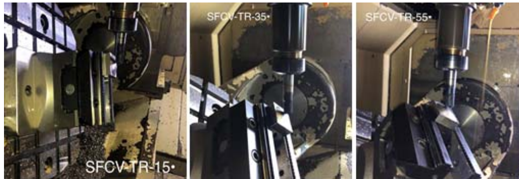
Fig. 4. Processing of the concave spherical surface with the toroidal milling machine in the case of the 3 types of inclinations
