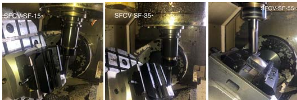
Fig. 5. Processing of the concave spherical surface with the spherical mill in the case of the 3 types of inclinations
