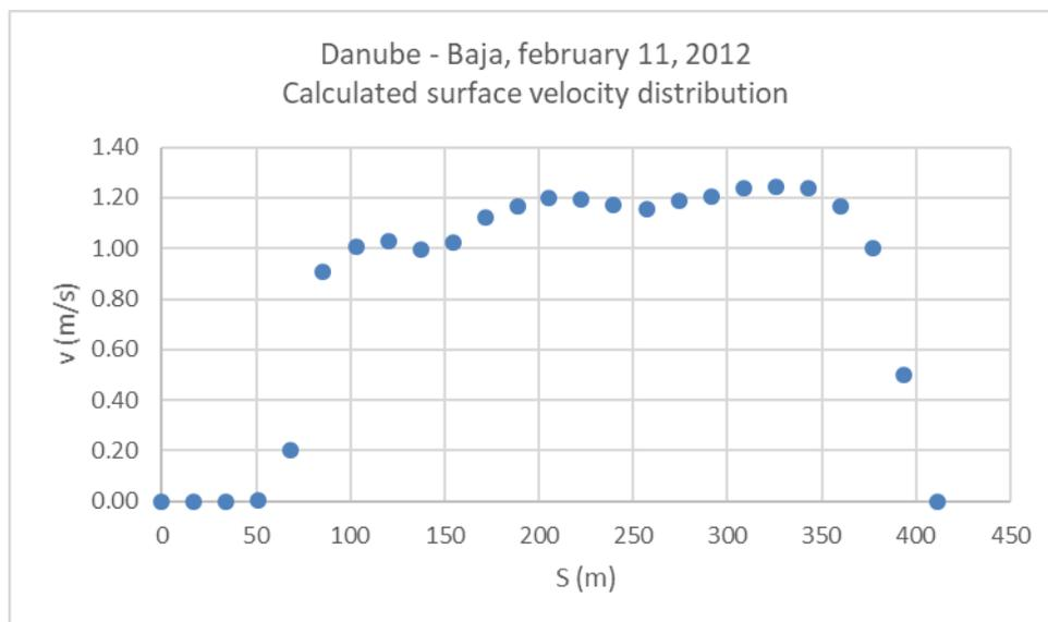
**Fig. 7.** Danube - Baja, february 11, 2012, Calculated surface velocity distribution
