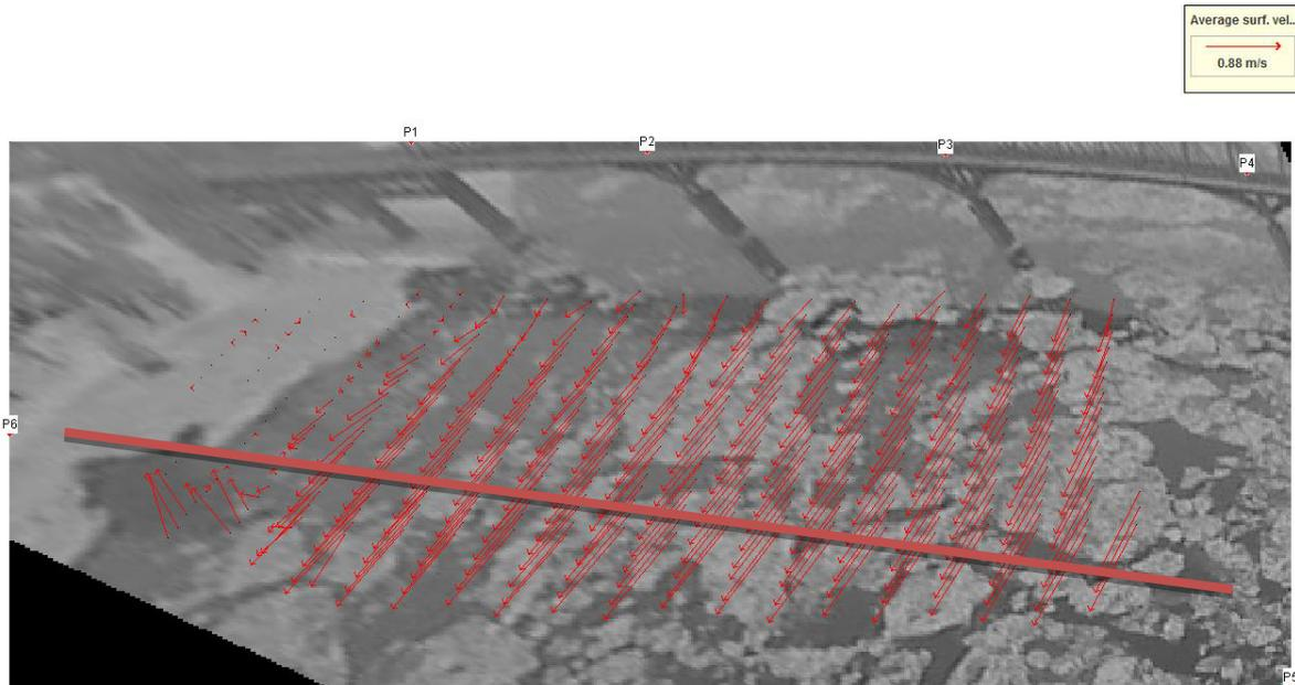
**Fig. 6.** Calculated LSPIV surface velocity field (Baja, Hungary, February 11, 2012)
