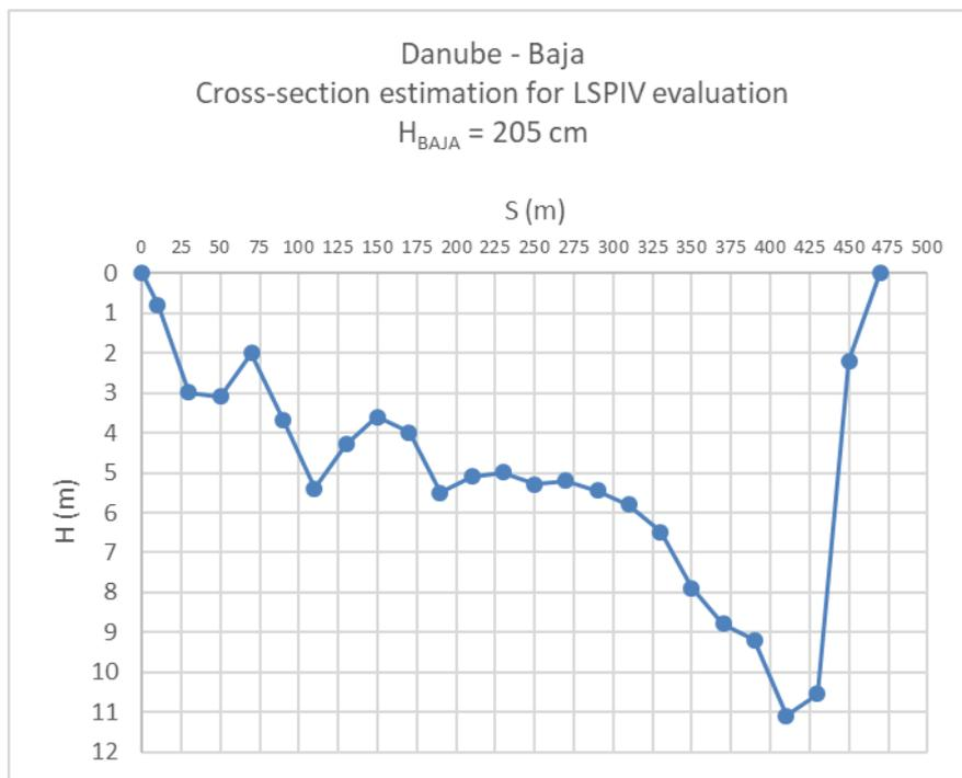
Fig. 9. Cross-section estimation for LSPIV evaluation, Danube - Baja
