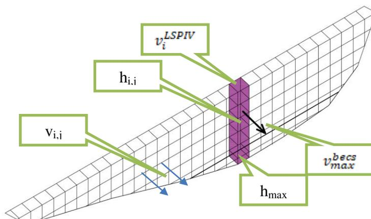
Fig. 3. Estimation of velocity distribution in a vertical profile
