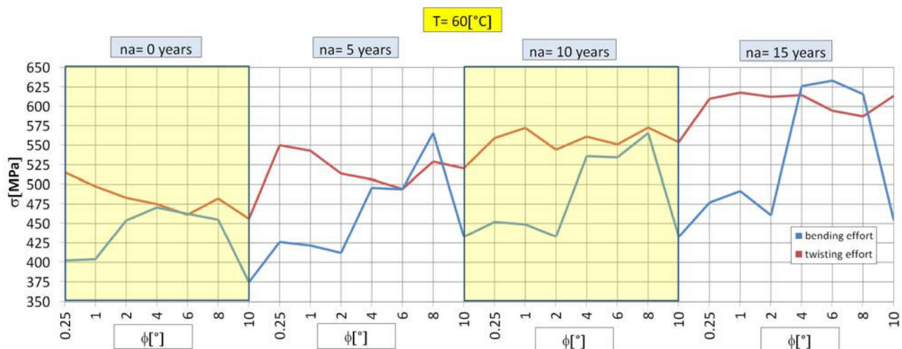
Fig. 10. The graphs of the Von Mises resultant efforts with highlighted details: ( T = 60\text{ }^{\circ}\text{C} ; n_a = \{0, 5, 10 \text{ and } 15 \text{ years}\} ; \phi = \{0.25^{\circ}, 1^{\circ}, 2^{\circ}, 4^{\circ}, 6^{\circ}, 8^{\circ} \text{ and } 10^{\circ}\} )
