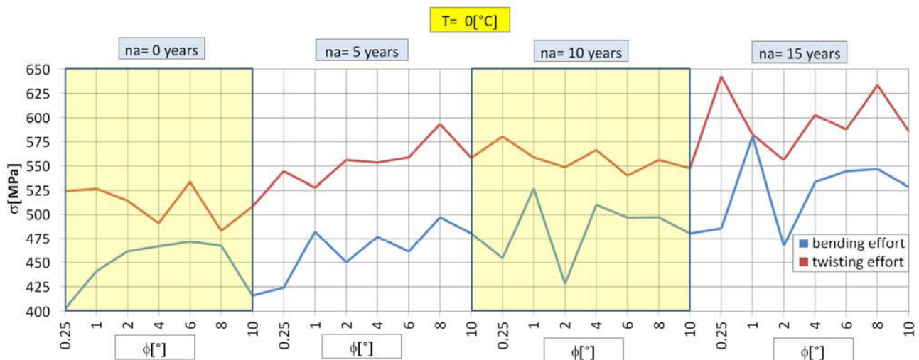
Fig. 12. The graphs of the Von Mises resultant efforts with highlighted details: ( T = 0\text{ }^{\circ}\text{C} ; n_a = \{0, 5, 10 \text{ and } 15 \text{ years}\} ; \phi = \{0.25^{\circ}, 1^{\circ}, 2^{\circ}, 4^{\circ}, 6^{\circ}, 8^{\circ} \text{ and } 10^{\circ}\} )
