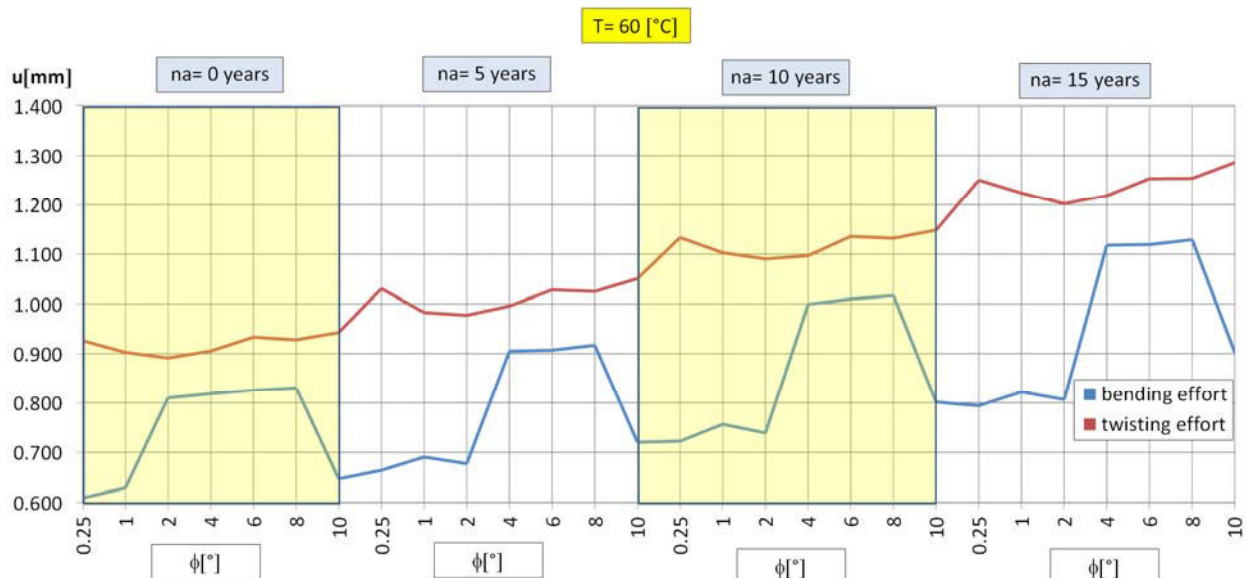
Fig. 19. The graphs of the variation of the resulting linear deformations u with highlighted details: (T = 60\text{ }^{\circ}\text{C}; n_a = \{0, 5, 10 \text{ and } 15 \text{ years}\}; \phi = \{0.25^{\circ}, 1^{\circ}, 2^{\circ}, 4^{\circ}, 6^{\circ}, 8^{\circ} \text{ and } 10^{\circ}\})
