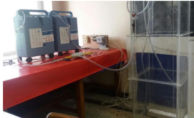
Fig. 3. Overview of the experimental installation for the introduction of a low nitrogen gas
