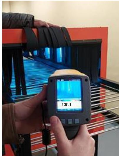
**Fig. 6.** Temperature measurement in the drying tunnel
