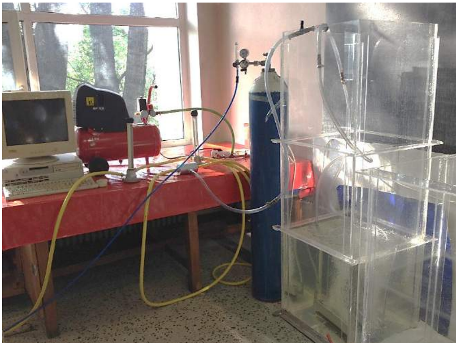
Fig. 2. Overview of the experimental installation for the introduction of a mixture of gases (atmospheric air and oxygen)
