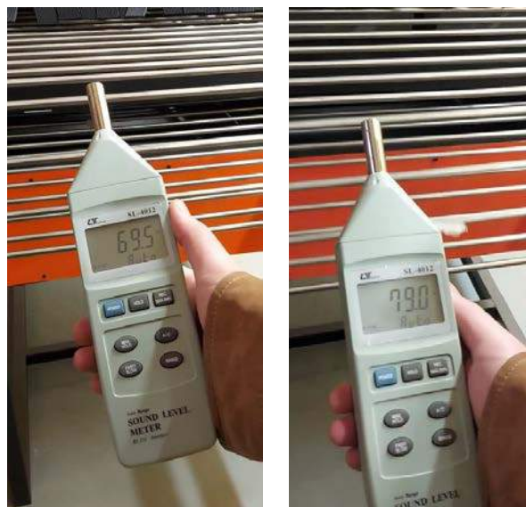
Fig. 5. Measurement / recording of vacuum vibration level with sound level meter model RS- 232:SL-4012
