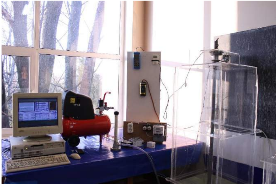
Fig. 3. Overview of the experimental installation for the introduction of atmospheric air
