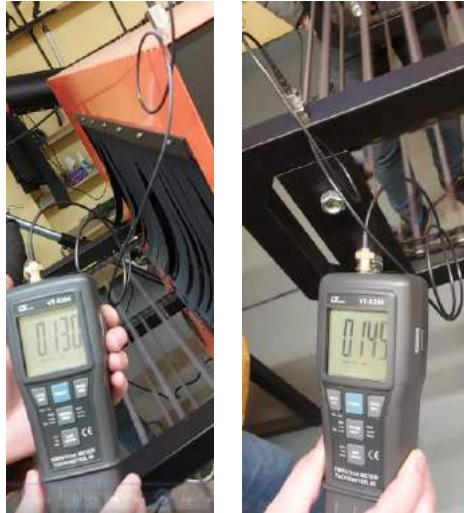
Fig. 4. Measurement / recording of vacuum vibration level with Lutron VT-8204
