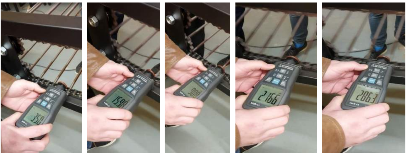
Fig. 3. Measuring the rotational speed of the conveyor belt
