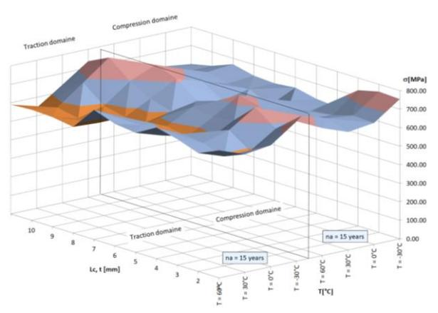
**Fig. 10.** The graphs of  $\sigma = f(L_c, T)$  for  $n_a = 15$  years left (traction area); right (compression area)
