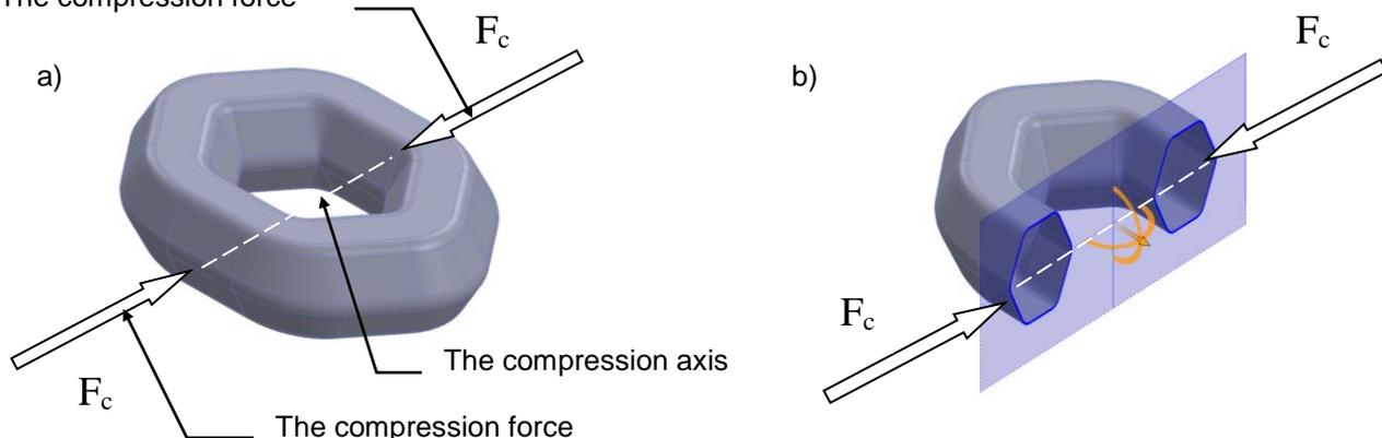
**Fig. 2.** The isometric representation of deformed 3-D model, after the uniaxial compression:
