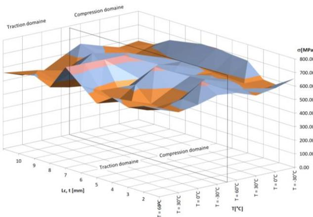
**Fig. 9.** The graphs of  $\sigma = f(L_c, T)$  for  $n_a = 10$  years left (traction domain); right (compression domain)
