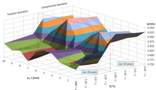
**Fig. 20.** The graphs of  $u = (L_c, T)$  for  $n_a = 15$  years left (traction area); right (compression area)
