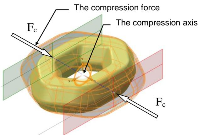
**Fig. 4.** The isometric representation of 3-D model, deformed, after the uniaxial compression
