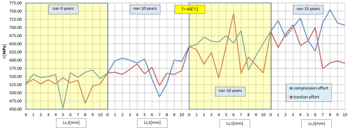
**Fig. 14.** The graphs of the Von Mises resultant efforts  $\sigma = f(L_c, T)$  with highlighted details: ( $T = 60\text{ }^\circ\text{C}$ ;  $n_a = \{0, 5, 10 \text{ and } 15\text{ years}\}$ ; blue curve – the compression effort; red curve – the traction effort.
