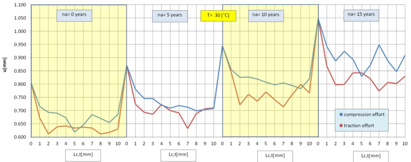
**Fig. 23.** The graphs of the resulting linear deformations  $u = f(L_c, T)$  with highlighted details: ( $T = 30\text{ °C}$ ;  $n_a = \{0, 5, 10 \text{ and } 15 \text{ years}\}$ ; blue curve – the compression effort; red curve – the traction effort;
