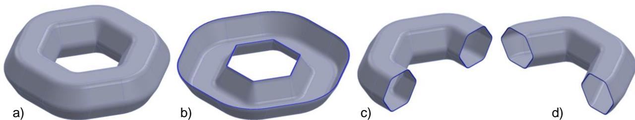
**Fig. 1.** The isometric representation of non-deformed 3-D model: a) view; b), c) and d) different sections
