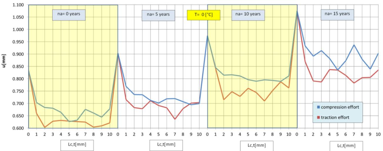
**Fig. 22.** The graphs of the resulting linear deformations  $u = f(L_c, T)$  with highlighted details: ( $T = 0$  °C;  $n_a = \{0, 5, 10$  and  $15$  years}; blue curve – the compression effort; red curve – the traction effort;
