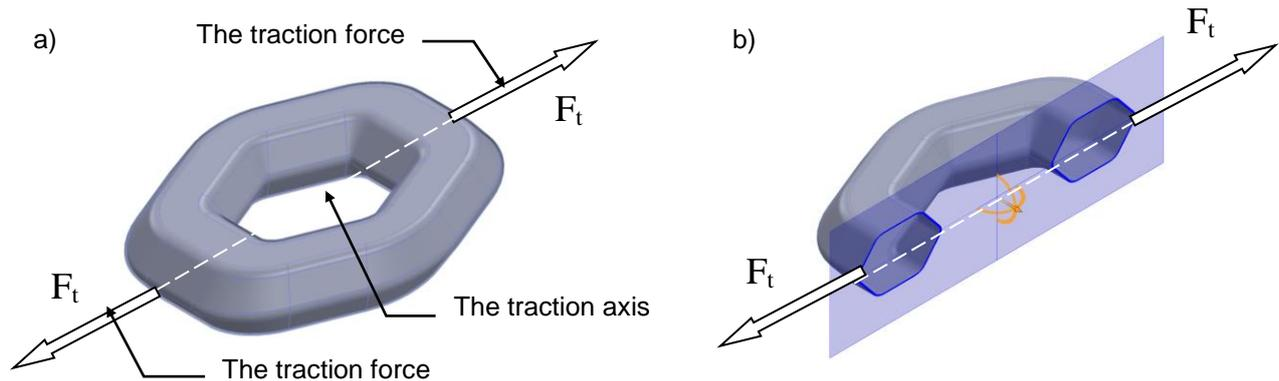
**Fig. 3.** The isometric representation of deformed 3-D model, after the uniaxial traction: a) view; b) cross section
