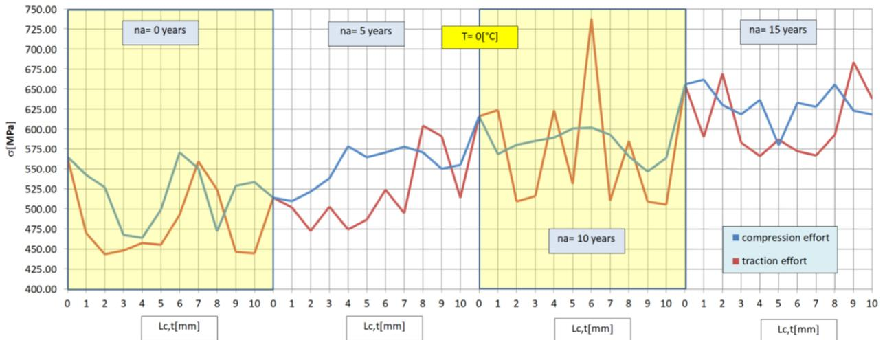
**Fig. 12.** The graphs of the Von Mises resultant efforts  $\sigma = f(L_c, T)$  with highlighted details: ( $T = 0\text{ }^\circ\text{C}$ ;  $n_a = \{0, 5, 10 \text{ and } 15 \text{ years}\}$ ; blue curve – the compression effort; red curve – the traction effort;
