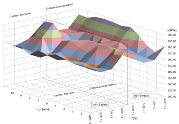
**Fig. 8.** The graphs of  $\sigma = f(L_c, T)$  for  $n_a = 5$  years left (traction area); right (compression area)
