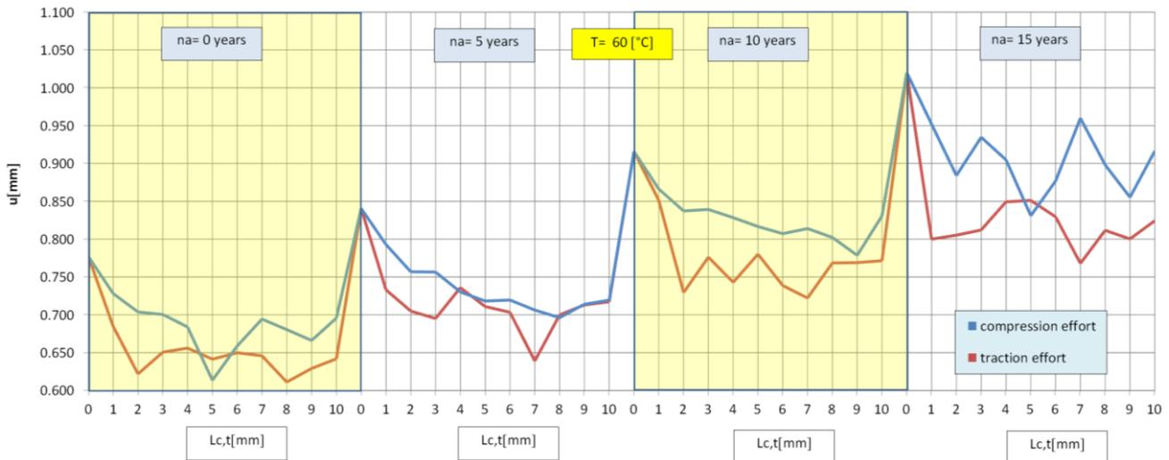
**Fig. 24.** The graphs of the resulting linear deformations  $u = f(L_c, T)$  with highlighted details: ( $T = 60\text{ °C}$ ;  $n_a = \{0, 5, 10 \text{ and } 15 \text{ years}\}$ ; blue curve – the compression effort; red curve – the traction effort;
