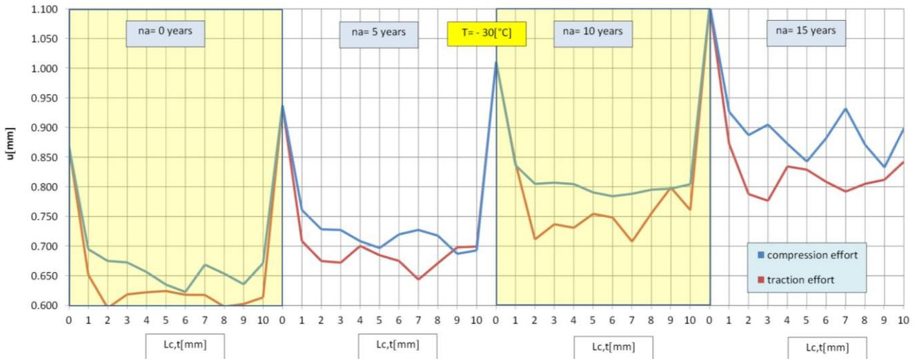
**Fig. 21.** The graphs of the resulting linear deformations  $u = f(L_c, T)$  with highlighted details: ( $T = -30$  °C;  $n_a = \{0, 5, 10$  and  $15$  years}; blue curve – the compression effort; red curve – the traction effort;
