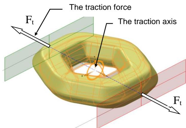
**Fig. 5.** The isometric representation of 3-D model, deformed, after the uniaxial traction
