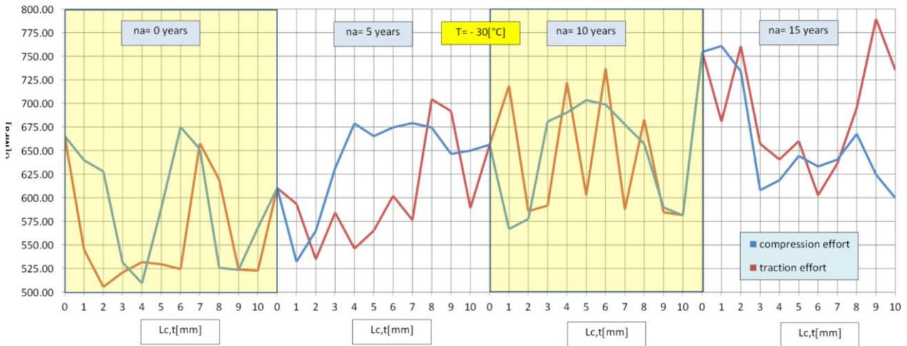
**Fig. 11.** The graphs of the Von Mises resultant efforts  $\sigma = f(L_c, T)$  with highlighted details: ( $T = -30\text{ }^\circ\text{C}$ ;  $n_a = \{0, 5, 10 \text{ and } 15 \text{ years}\}$ ; blue curve – the compression effort; red curve – the traction effort;
