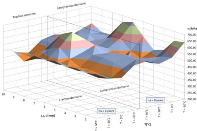
**Fig. 7.** The graphs of  $\sigma = f(L_c, T)$  for  $n_a = 0$  years left (traction domain); right (compression domain)
