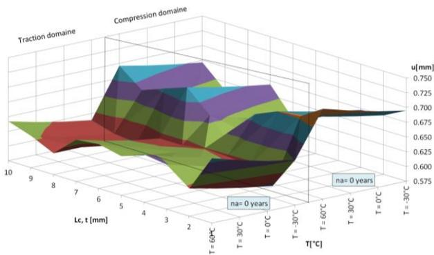
Fig. 17. The graphs of  $u = (L_c, T)$  for  $n_a = 0 \text{ years}$  left (traction domain); right (compression domain)
