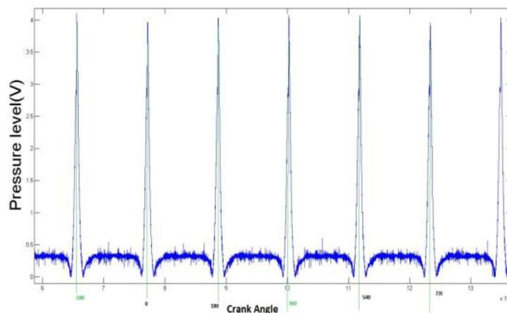
Fig. 2. Cylinder Pressure
