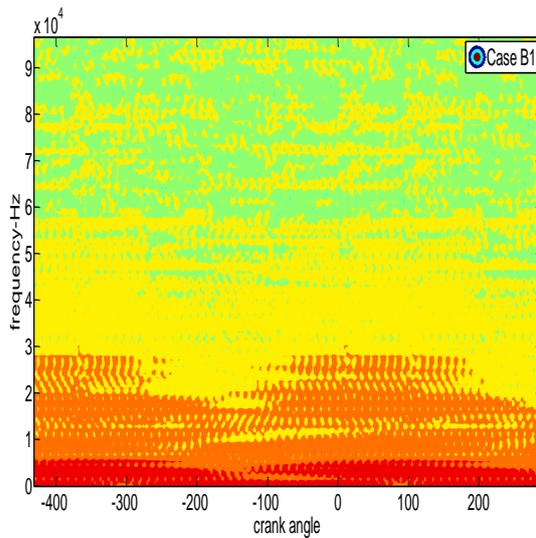
Fig. 11. CWT Time-Frequency plot(B1)
