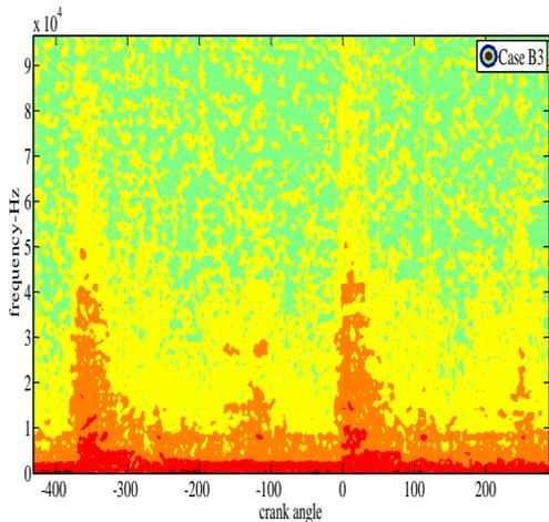
Fig. 5. Time-Frequency plot(B3)
