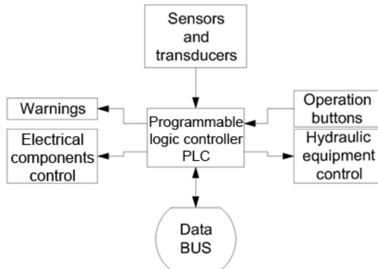
Fig. 2. Hardware structure of the data acquisition and control system of a designed test stand
