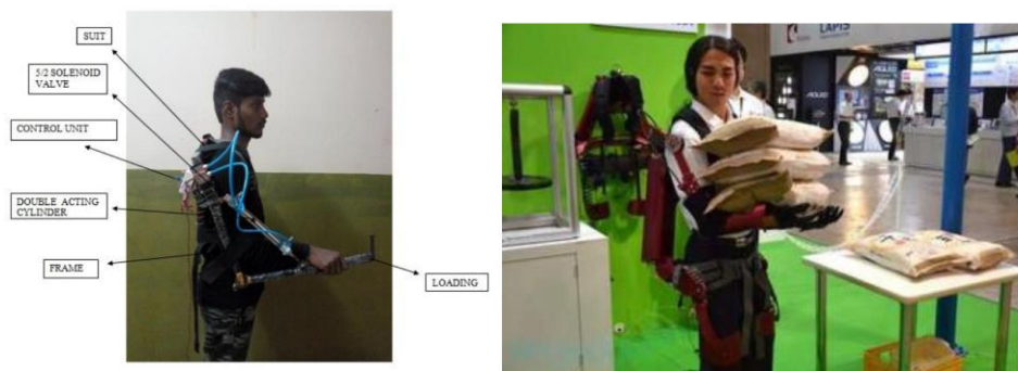
Fig. 7. Pneumatic exoskeletons for industrial use 0, 0
