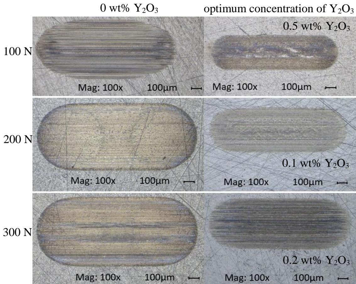
Fig. 6. Comparison of the wear scars on the disc specimen using digital microscopic images
