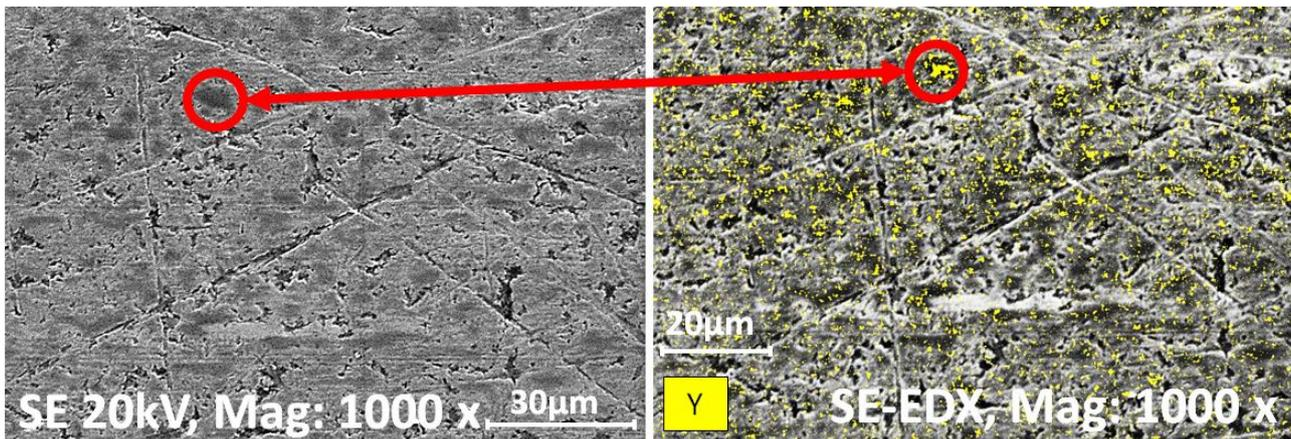
**Fig. 7.** SE-Scanning Electron Microscope image and EDX mapping picture about the surface of disc specimen with 0.5 wt%  $Y_2O_3$  doped Gr III base oil
