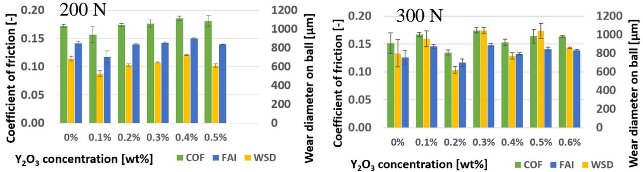
Fig. 5. Comparison of the experimental results of analyzed 0W-20-based lubricant samples with various nanoparticle concentration under 200 N (left) and 300 N (right) load
