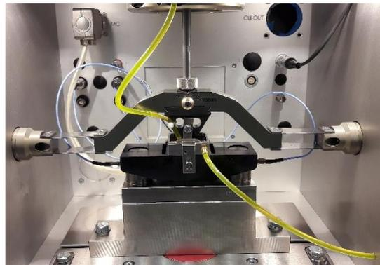
**Fig. 2.** The used Optimol SRV®5 tribometer with the installed pipes of the oil circuit
