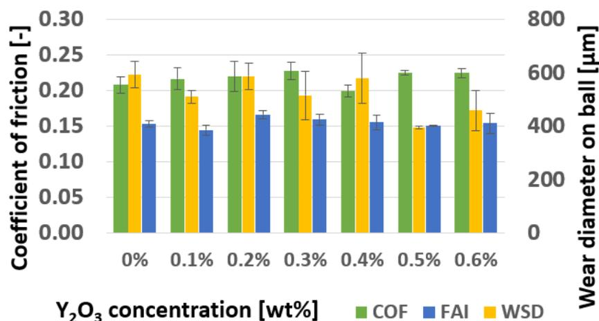
Fig. 4. Comparison of the experimental results of analyzed Gr III-based lubricant samples with various nanoparticle concentration
