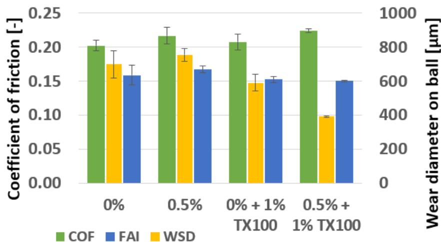
Fig. 3. Comparison of the tribological results with triton-doped and non-triton doped oil samples
