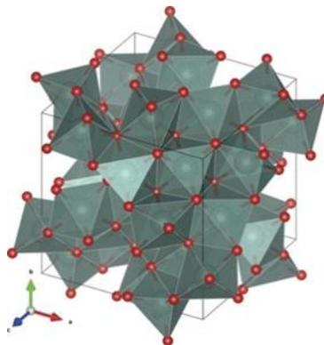
Fig. 1. Body-centered cubic crystal structure of  $Y_2O_3$  [5]
