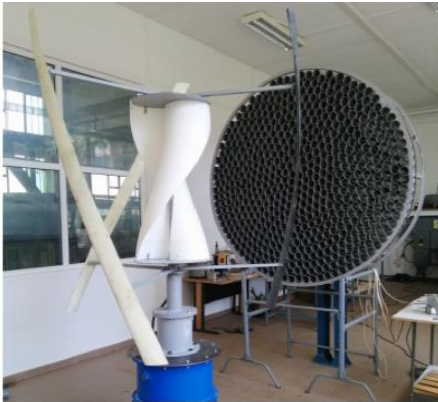
Fig. 11. Experimental model of the Darrieus + Savonius hybrid vertical-axis wind turbine
