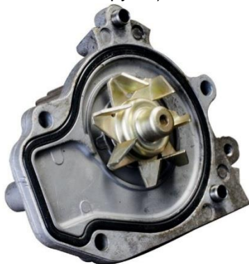
c) Car cooling pump
