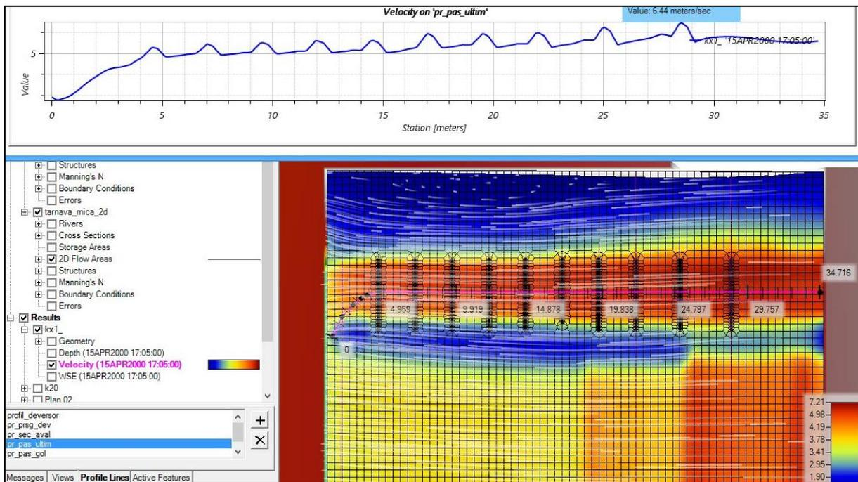
Fig. 12. Particles trajectories overlaid to water velocity spectrum together with velocity longitudinal unfolding by the fish passage middle line, at the specific moment when the maximum flow (408.50m³/s) is discharged
