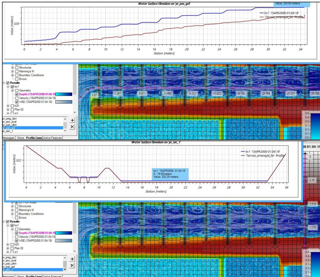
**Fig. 8.** Particles trajectories overlaid to water depth together with water surface longitudinal unfolding by the fish passage rows gaps and transverse profile by the first upstream three stones row of the side passage, at the specific moment when the sanitary flow ( $2.48\text{m}^3/\text{s}$ ) is discharged
