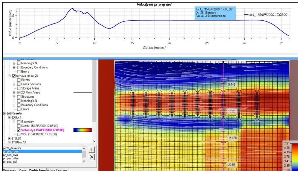
Fig. 13. Particles trajectories overlaid to water velocity spectrum together with velocity entire transverse profile by the second step, at the specific moment when the maximum flow ( $408.50\text{m}^3/\text{s}$ ) is discharged
