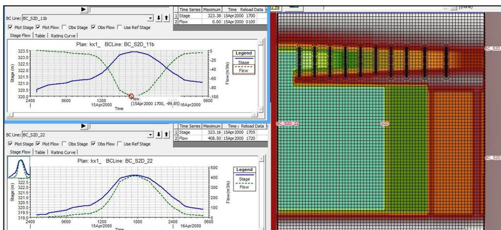
Fig. 14. Correlated water flow and level time development by the fish passage entrance (above) and entire arrangement outgoing borders of the Târnava Mică River modeled sector
