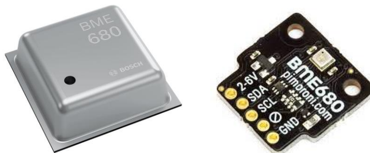
Fig. 2. BME 680 Bosch air quality sensor [9]
