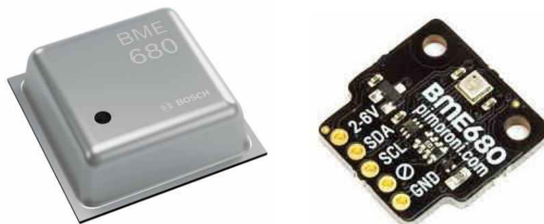
Fig. 2. BME 680 Bosch air quality sensor [9]
