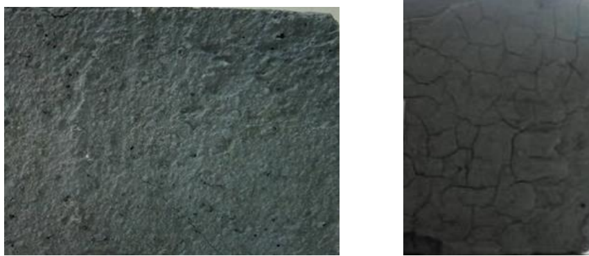
Fig. 5. Brick obtained from mud and cement [14]
