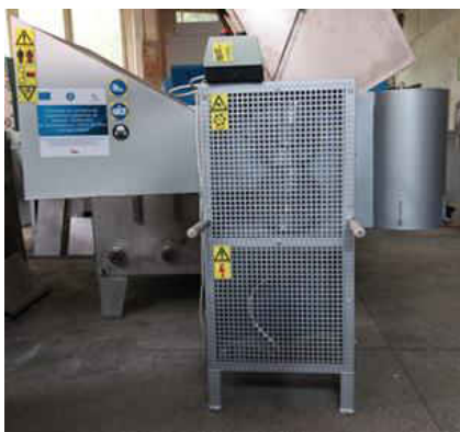
Fig. 3. Chopper driven with electric engine of 2.2 kW
