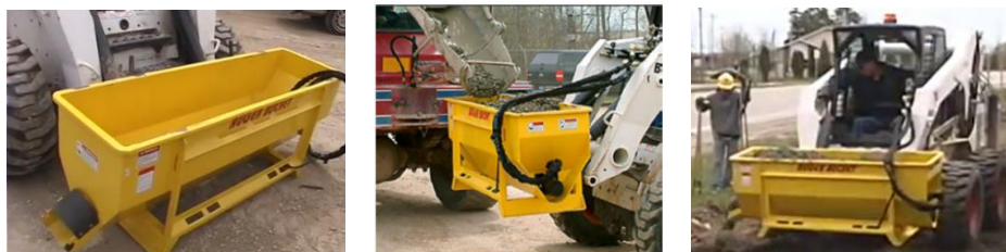
Fig. 1. Working principle of the mixing bucket for loader [2]
