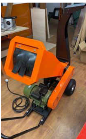
Fig. 4. Shredder driven with electric engine of 4 kW
