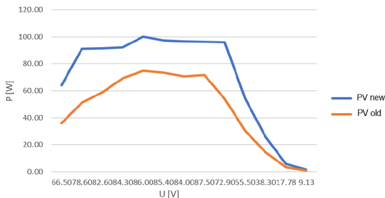
Fig. 6. The output power for a new and old panel
