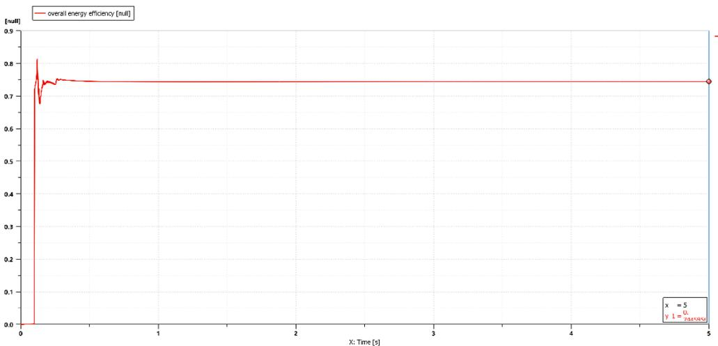
**Fig. 11.** Time variation of the overall energy efficiency of the closed circuit hydrotronic transmission
