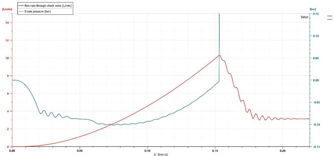
Fig. 4. Detail - Main pump suction port pressure variation and compensation flow rate
