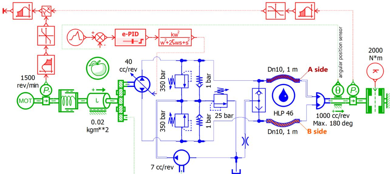
**Fig. 2.** Simulation network - hydrotronic transmission
