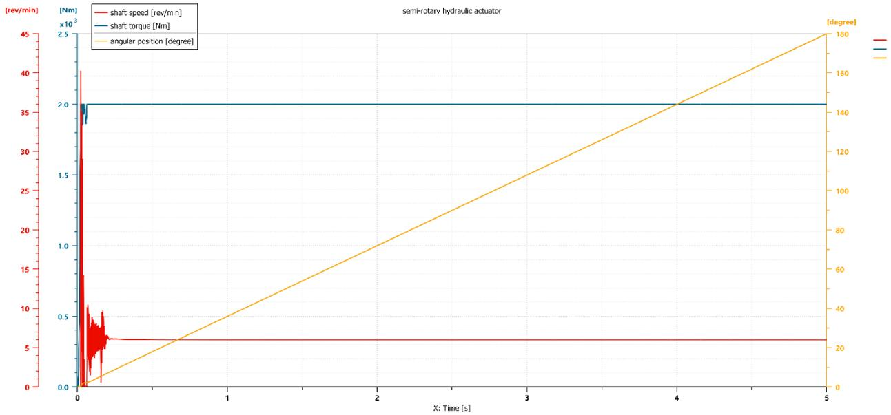
**Fig. 7.** Time variation of the parameters of the semi-rotary hydraulic actuator
