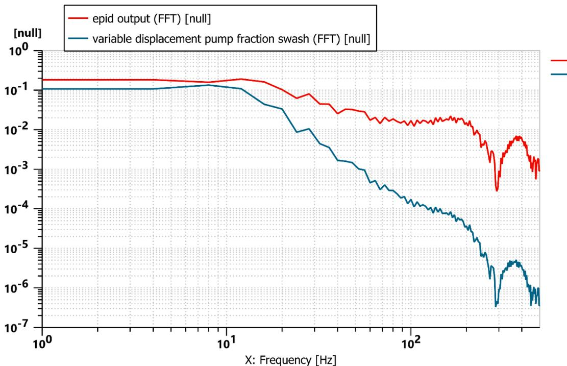
Fig. 6. Frequency spectrum of the PID controller output signal comparative to pump fraction swash
