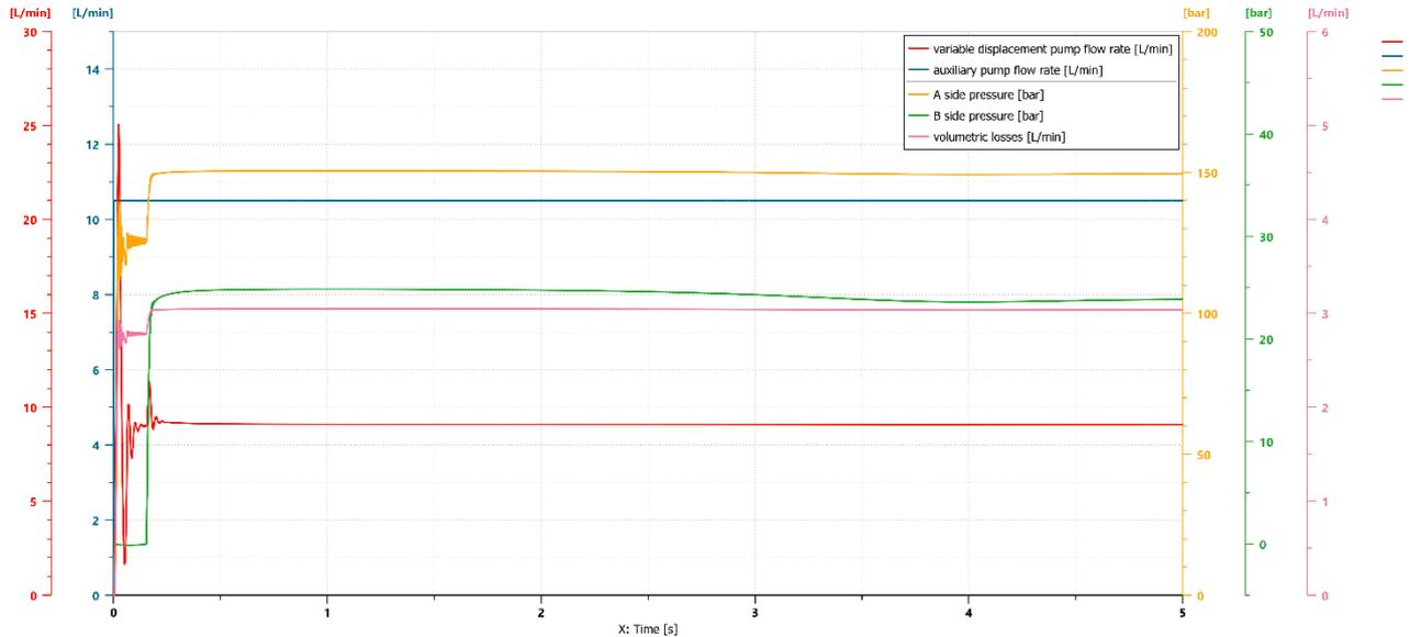
Fig. 3. Time variation of system pressures and flow rates
