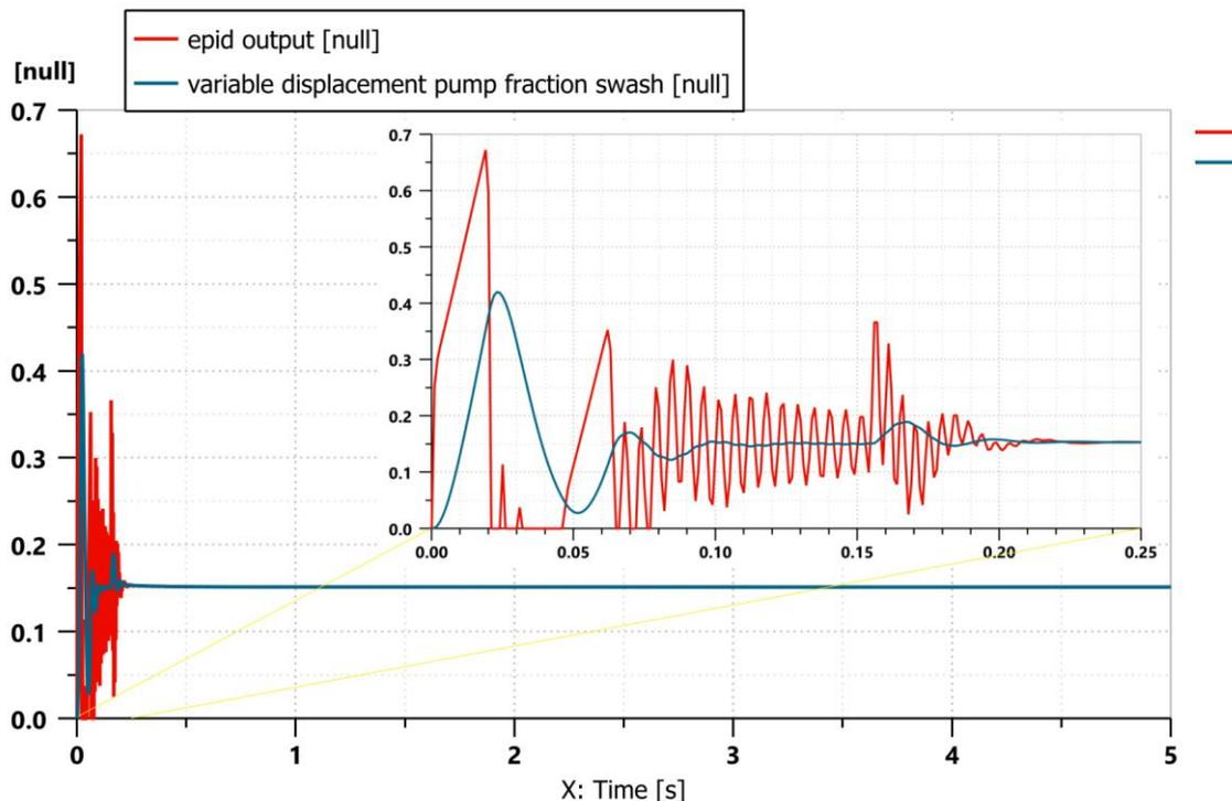
Fig. 5. Time variation of the PID controller output and the pump fraction swash
