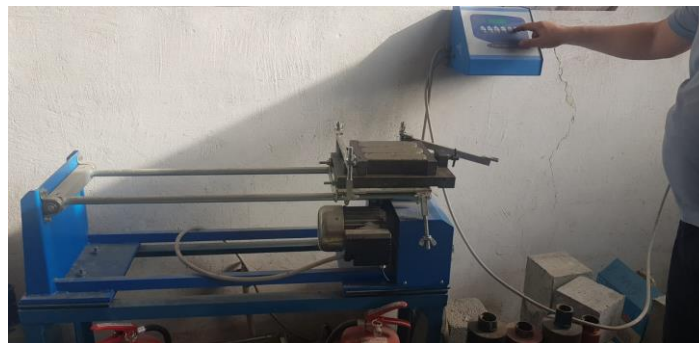
Fig. 6. Compaction by mechanical shocks
