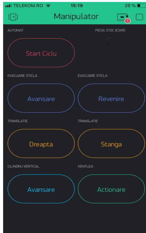
Fig. 7. Virtual control panel in the Blynk app
