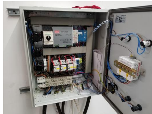
Fig. 7. The electric cabinet for the bench and electric motor control
