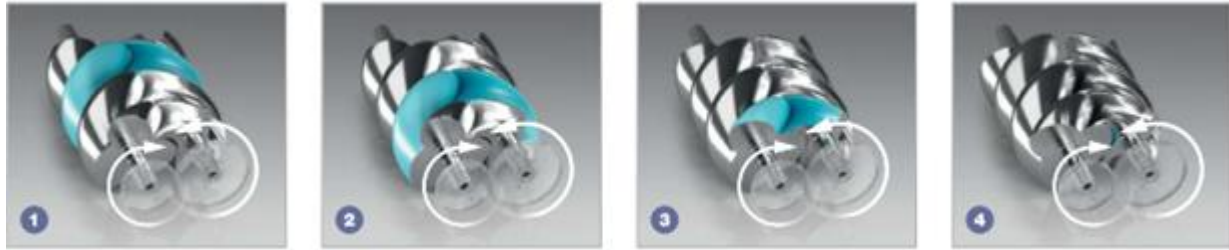
Fig. 1. Air flow through a screw blower [4]
