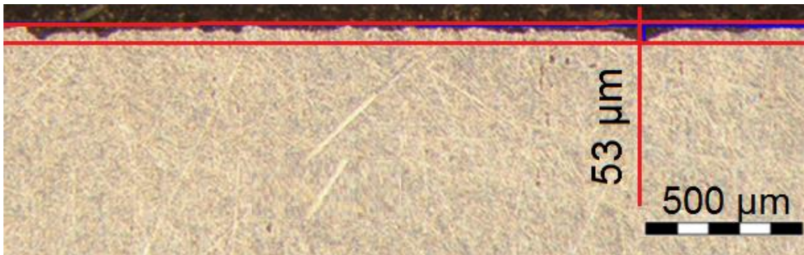
a) Microscopic image measuring the depth of a cavern in the eroded area
