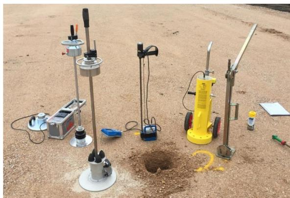
Fig. 2. Usual devices for in-situ measurements of the terrain properties with: Light Weight Deflectometer, Dynamic Cone Penetrometer, Clegg Hammer, Plate Load Testing.
