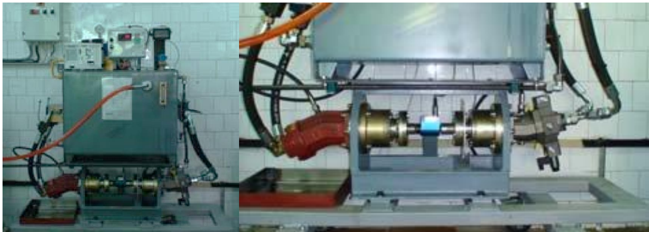
Fig. 7. Experimental stand for the study of the closed-loop transmission with secondary adjustment
