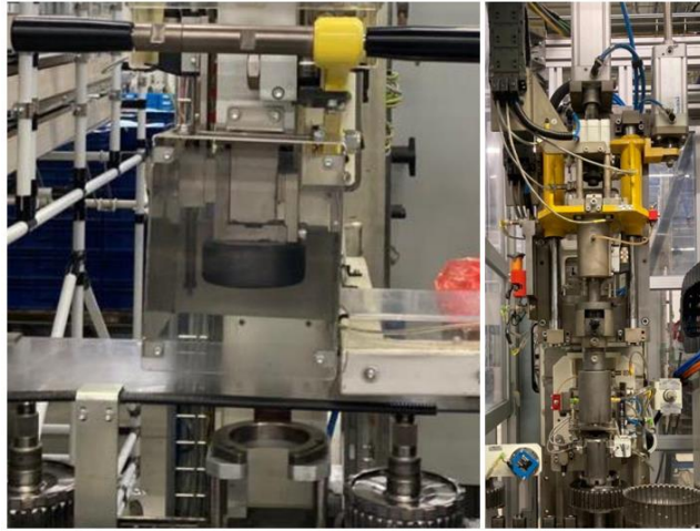
Fig. 1. Mechanised vs automated (pneumatic) bearing pressing station
