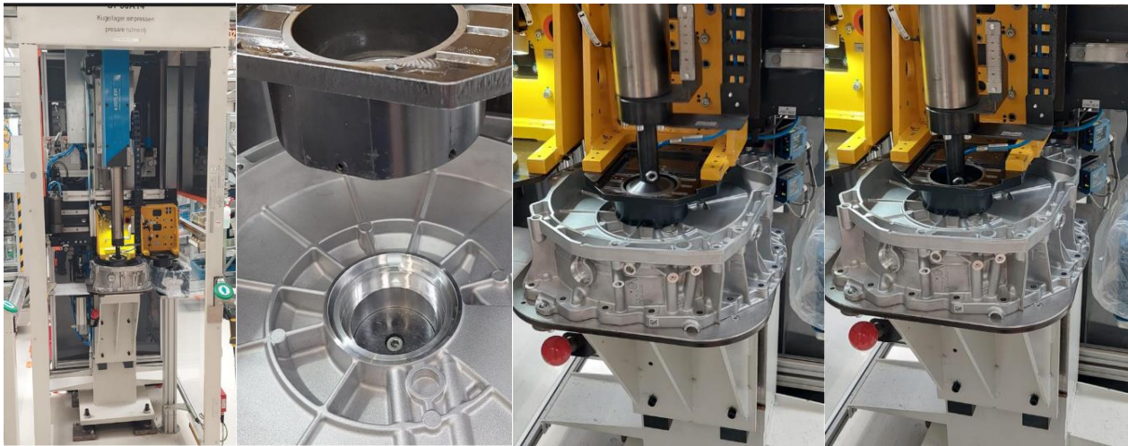
Fig. 6. Pressing station after modification/ Port bearing piece/ Starting and ending of the pressing process
