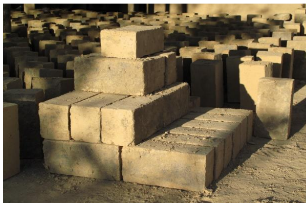
Fig. 7. Drying of bricks in special halls [12]
