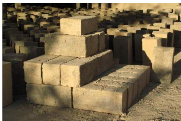
Fig. 7. Drying of bricks in special halls [12]
