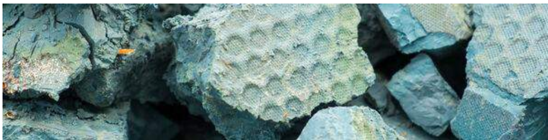
Fig. 2. The cake produced by the press filter, which has chunks of dehydrated sludge solids with an imprint of the filter cell membrane [8]
