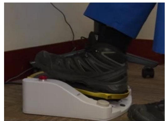
Fig. 10. The pedal used by the surgeon from New York to control the robot's positions [9]
