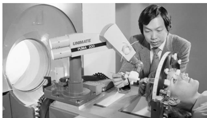
Fig. 1. PUMA 200, the first robot used to assist human neurosurgery [2]
