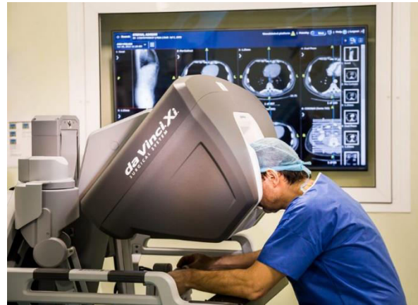
Fig. 4. The console through which the surgeon controls the da Vinci Xi robot [3]
