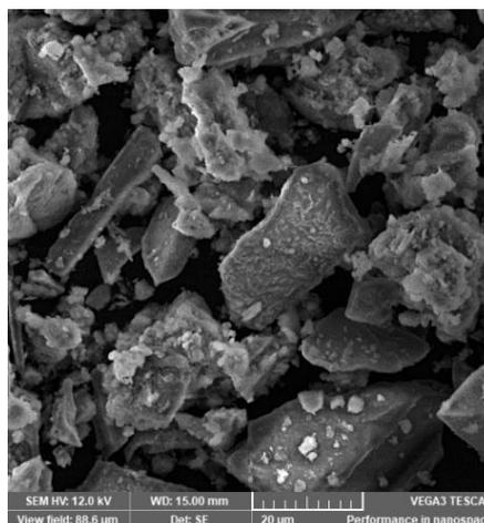
**Fig. 2.** SEM images of the NZ1 200 zeolite sample
