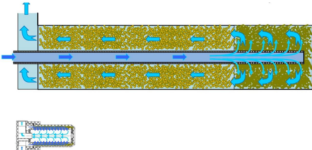
**Fig. 1.** Design of the natural zeolites-based filter for water filtration
