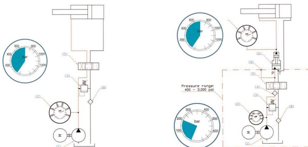
Fig. 1. Generating a pressure of 700 bar for actuating a hydraulic cylinder: left - with high-pressure pump; right - with low-pressure pump and hydraulic intensifier
