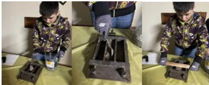
Fig. 3. Pouring and compacting the mixture
