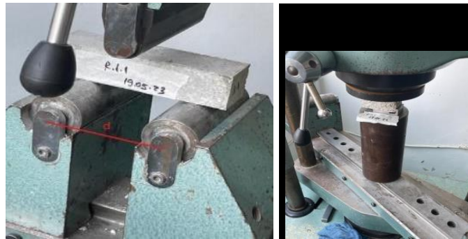
Fig. 5. Mechanical tests: a) tensile bending test, b) compression test
