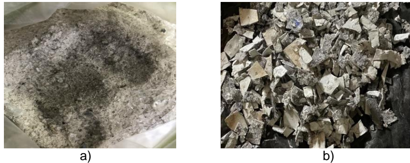
Fig. 1. The final materials obtained: a) PV dust (PVd), b) PV pieces (glass+plastic)-PVp
